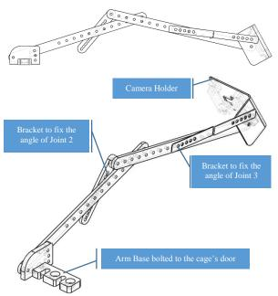
Figure 4: 2D and isometric drawing of a Camera Arm
