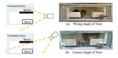
Figure 3: Modifying the cameras' angle of view to capture the cat when it is in close contact with the food
