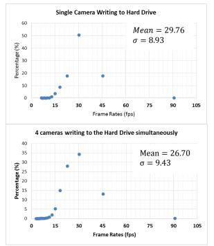
Figure 7: Frame rates versus the percentage of the total frames that were recorded. The system was tested in Intel i5 Processor with 8 GB RAM and 7200 RPM Hard Drive.
