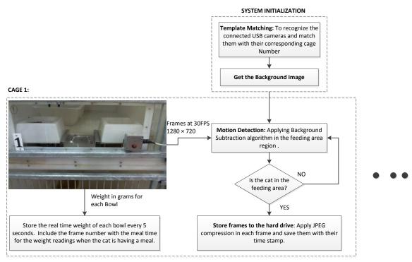
Figure 1: Block diagram of the real time monitoring of cat feeding behaviour system
