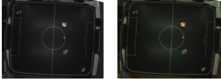
Fig. 3. Left: Raw image captured from the camera, Right: after Bayer interpolation
