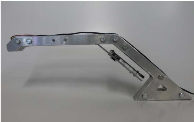
Figure 1: Setup showing FPGA camera on right with laser cantilevered on the left
